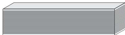
127 layer HSHT Filled Beam: (not to scale) 2 layers Nylon, 125 layers HSHT Glass CFF: Heat Deflection: 150 °C
